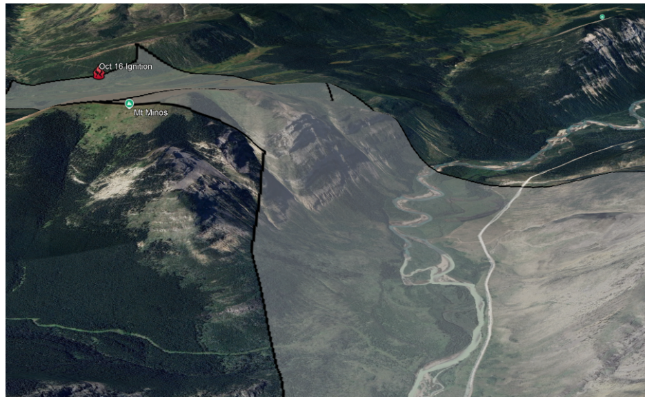
Figure 4.7: The 60 degree downhill part of fire spread shown in Google Earth. It is highly likely that the fire spread of the real fire was assisted and accelerated by firebrands travelling from the top of the hill to the valley below and beyond the river. However, firebrand-assisted propagation is already reflected in the CFFDRS spread rate regressions, and as such should not be activated in ELMFIRE.
